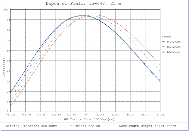
#15-648, 25mm, f/2.8 Cw Series Fixed Focal Length Lens, Depth of Field Plot, 500mm Working Distance, f2.8
