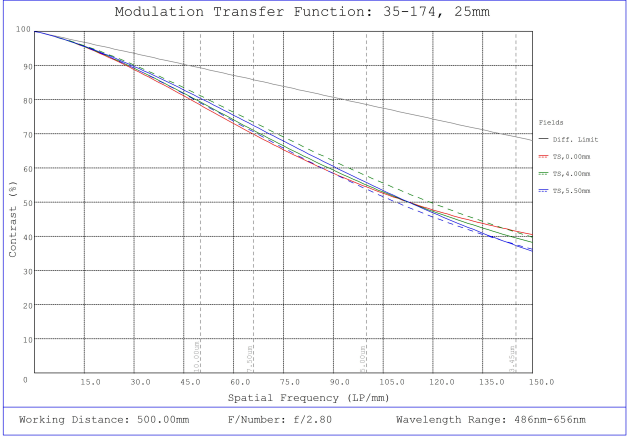
#35-174, 25mm, f/2.8 Cr Series Fixed Focal Length Lens, Modulated Transfer Function (MTF) Plot, 500mm Working Distance, f2.8
