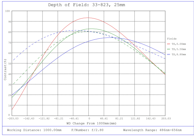
#33-823, 25mm f/2.8, HPI Series Fixed Focal Length Lens, Depth of Field Plot, 1000mm Working Distance, f2.8
