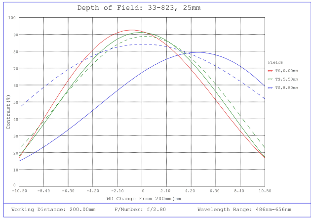
#33-823, 25mm f/2.8, HPI Series Fixed Focal Length Lens, Depth of Field Plot, 200mm Working Distance, f2.8
