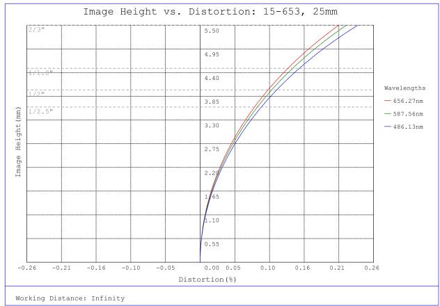
#15-653, 25mm, f/16 Cw Series Fixed Focal Length Lens, Distortion Plot
