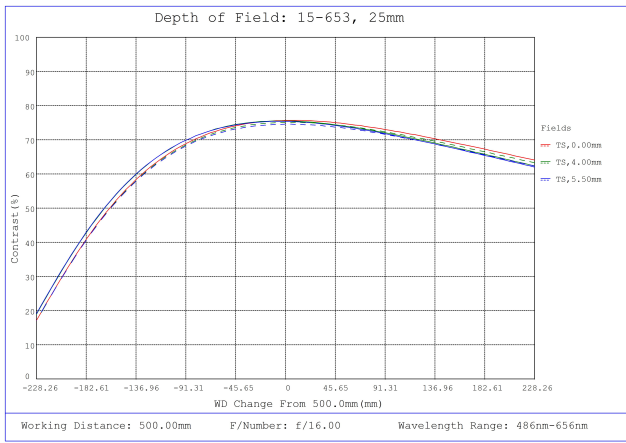
#15-653, 25mm, f/16 Cw Series Fixed Focal Length Lens, Depth of Field Plot, 500mm Working Distance, f16
