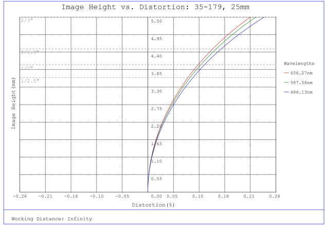
#35-179, 25mm, f/16 Cr Series Fixed Focal Length Lens, Distortion Plot
