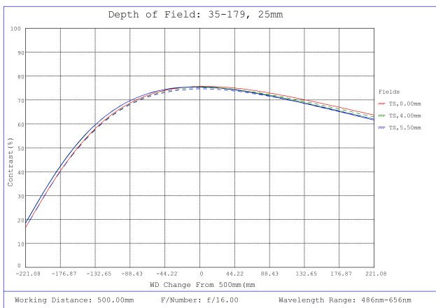
#35-179, 25mm, f/16 Cr Series Fixed Focal Length Lens, Depth of Field Plot, 500mm Working Distance, f16
