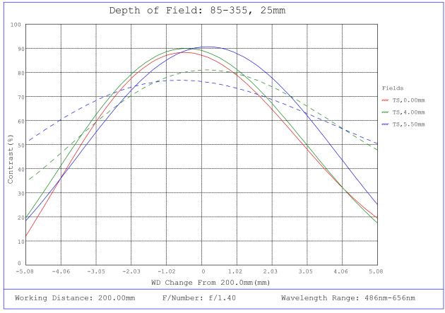
#85-355, 25mm, f/1.4 Ci Series Fixed Focal Length Lens, Depth of Field Plot, 200mm Working Distance, f1.4
