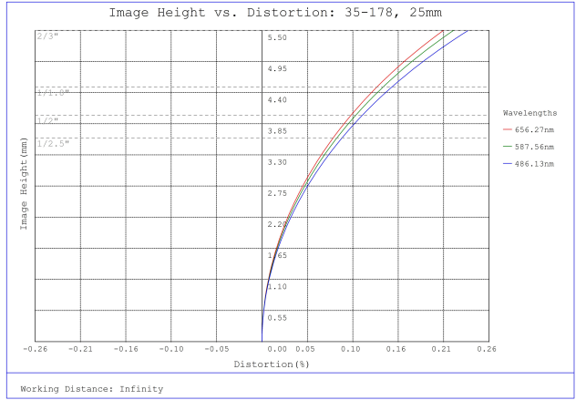
#35-178, 25mm, f/11 Cr Series Fixed Focal Length Lens, Distortion Plot
