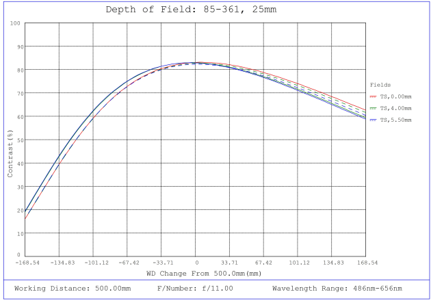
#85-361, 25mm, f/11 Ci Series Fixed Focal Length Lens, Depth of Field Plot, 500mm Working Distance, f11
