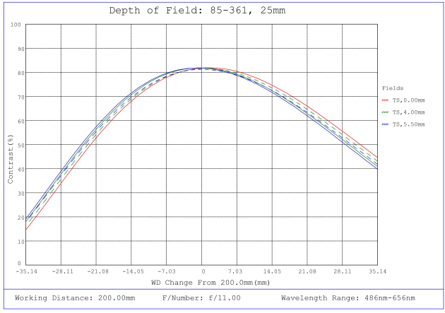
#85-361, 25mm, f/11 Ci Series Fixed Focal Length Lens, Depth of Field Plot, 200mm Working Distance, f11
