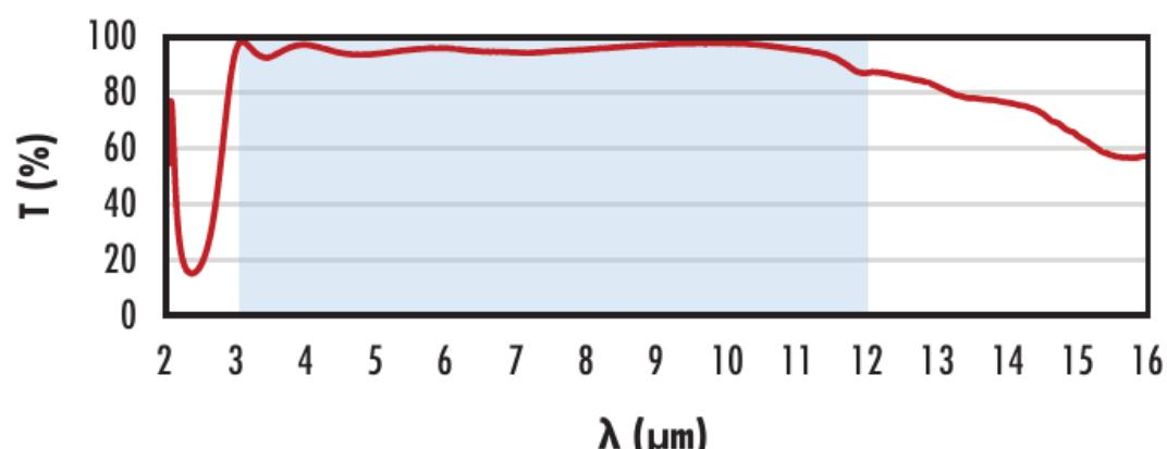
Typical transmission of a 3mm thick Ge window with BBAR (3000-12000nm) coating at 0° AOI.
