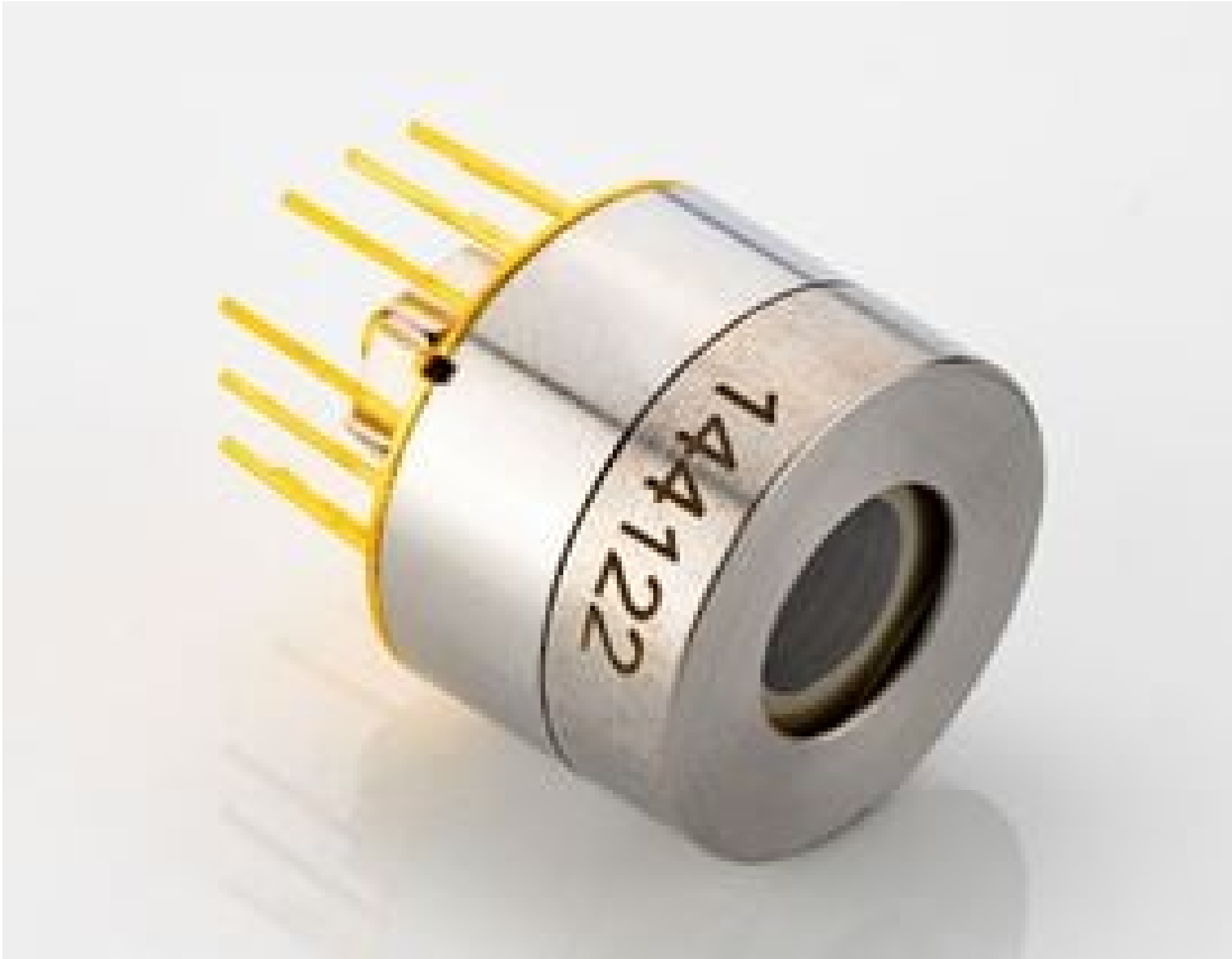
2.3 - 4.4um HgCdTe Photovoltaic Infrared Detector, PVI-2TE-4-1x1-TO8-wAl203-36
