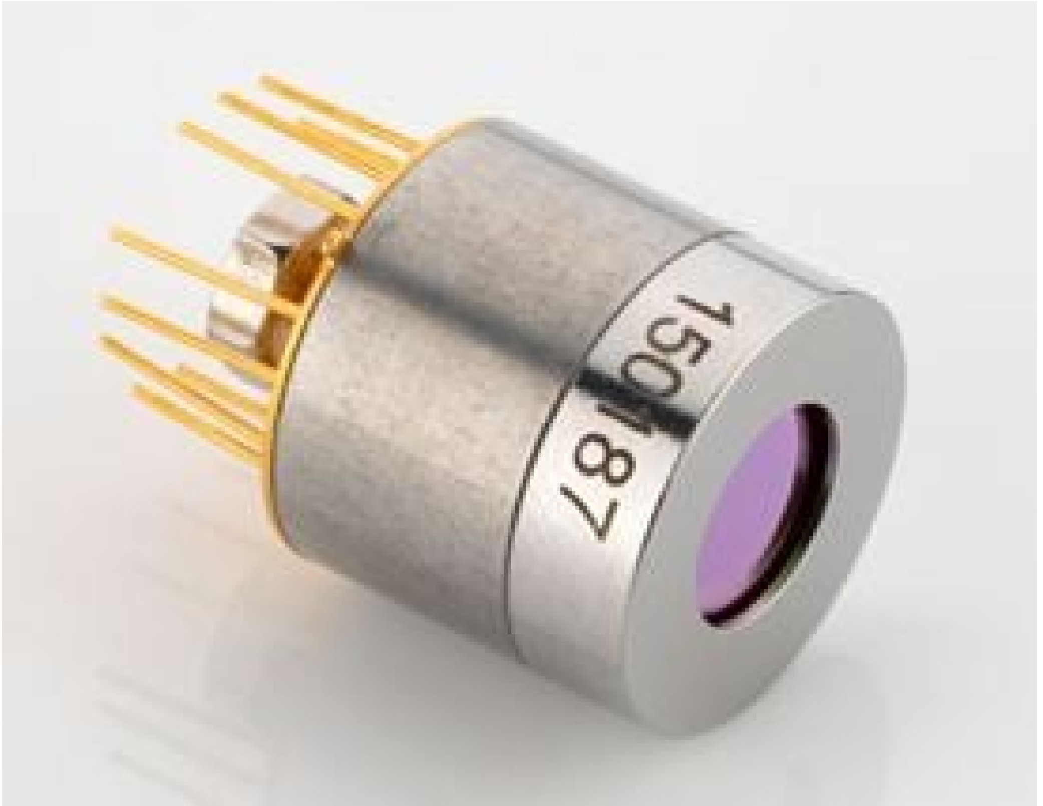
2.2 - 13.6 \mu\text{m} InAsSb Photovoltaic Infrared Detector, PVA-4TE-13-1 \times 1-TO8-wZnSeAR36
