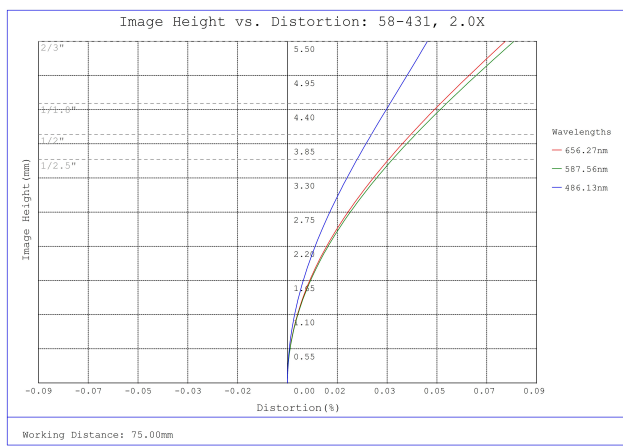
#58-431, 2.0X SilverTL™ Telecentric Lens, Distortion Plot
