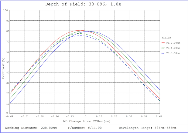
#33-096, 1X, 220mm WD CompactTL™ Telecentric Lens, Depth of Field Plot, 220mm Working Distance, f11
