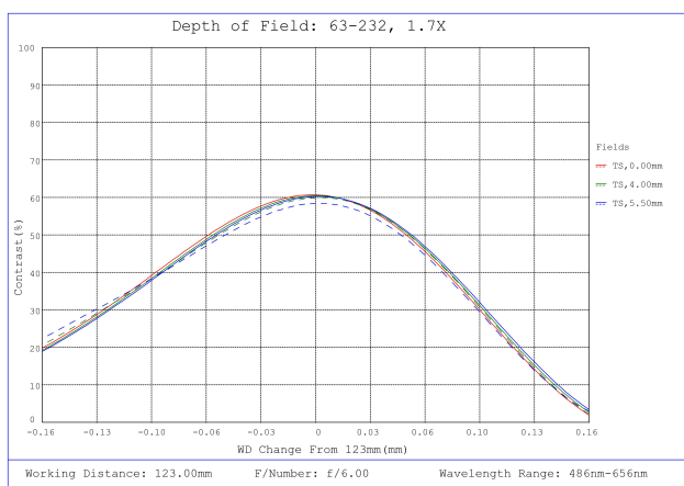
#63-232, 1.7X, 2/3" C-Mount PlatinumTL™ Telecentric Lens, Depth of Field Plot, 123mm Working Distance, f6
