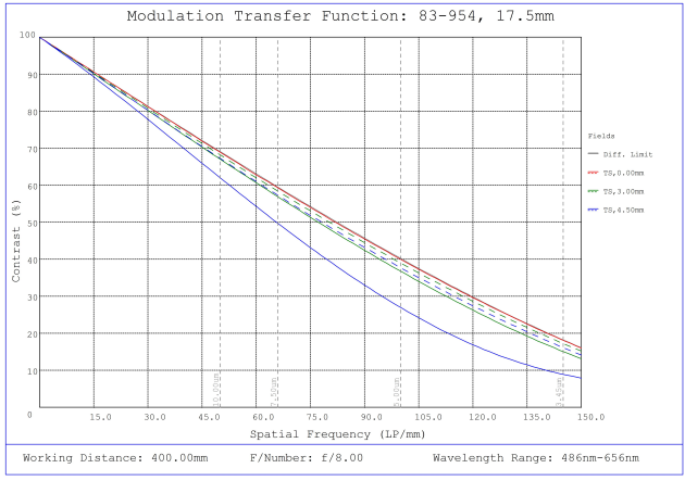
#83-954, 17.5mm FL f/8, Blue Series M12 Lens, Modulated Transfer Function (MTF) Plot, 400mm Working Distance, f8
