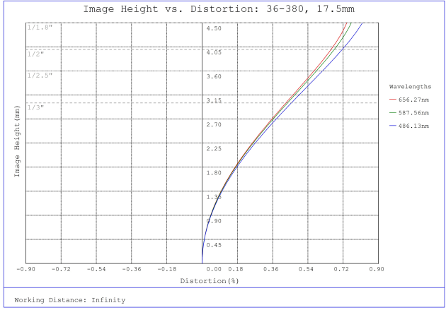
#36-380, 17.5mm FL f/2.5, Rugged Blue Series M12 Lens, Distortion Plot
