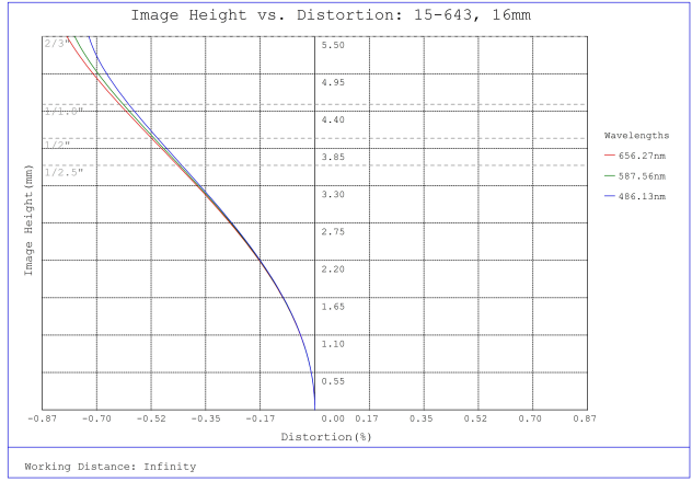
#15-643, 16mm, f/8 Cw Series Fixed Focal Length Lens, Distortion Plot
