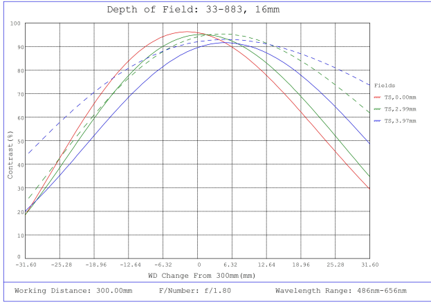
#33-883, 16mm, f/1.8 UCI Series Fixed Focal Length Lens, Depth of Field Plot, 300mm Working Distance, f1.8
