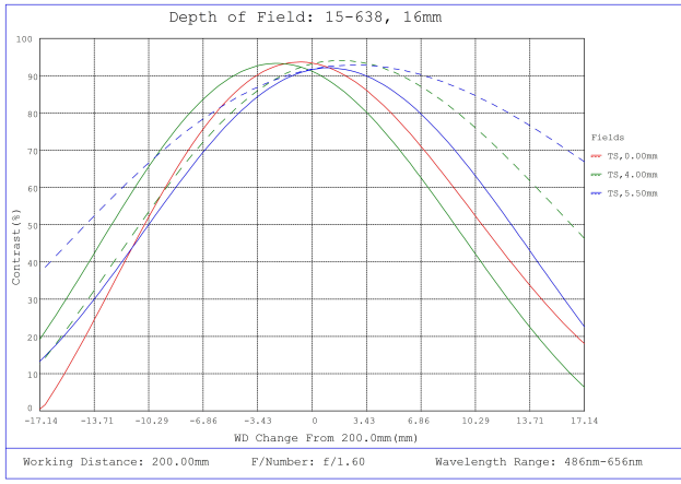
#15-638, 16mm, f/1.6 Cw Series Fixed Focal Length Lens, Depth of Field Plot, 200mm Working Distance, f1.6
