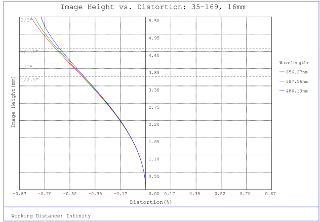
#35-169, 16mm, f/11 Cr Series Fixed Focal Length Lens, Distortion Plot
