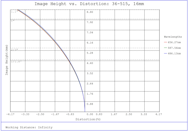
#36-515, 16mm f/8, HPr Series Fixed Focal Length Lens, Distortion Plot
