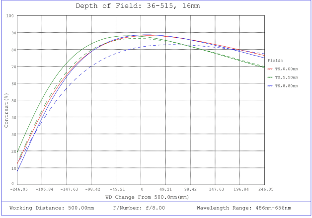
#36-515, 16mm f/8, HPr Series Fixed Focal Length Lens, Depth of Field Plot, 500mm Working Distance, f8
