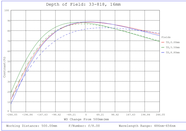
#33-818, 16mm f/8, HPI Series Fixed Focal Length Lens, Depth of Field Plot, 500mm Working Distance, f8
