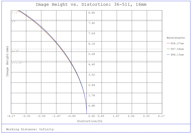
#36-511, 16mm f/1.8, HPr Series Fixed Focal Length Lens, Distortion Plot
