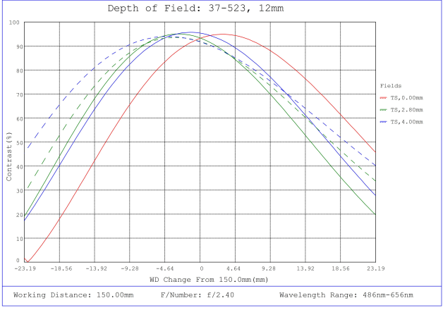
#37-523, 12mm FL, Liquid Lens M12 Lens, Depth of Field Plot, 150mm Working Distance, f2.4
