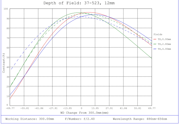
#37-523, 12mm FL, Liquid Lens M12 Lens, Depth of Field Plot, 300mm Working Distance, f2.4
