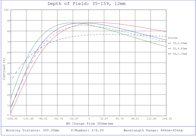
#35-159, 12mm, f/8 Cr Series Fixed Focal Length Lens, Depth of Field Plot, 300mm Working Distance, f8
