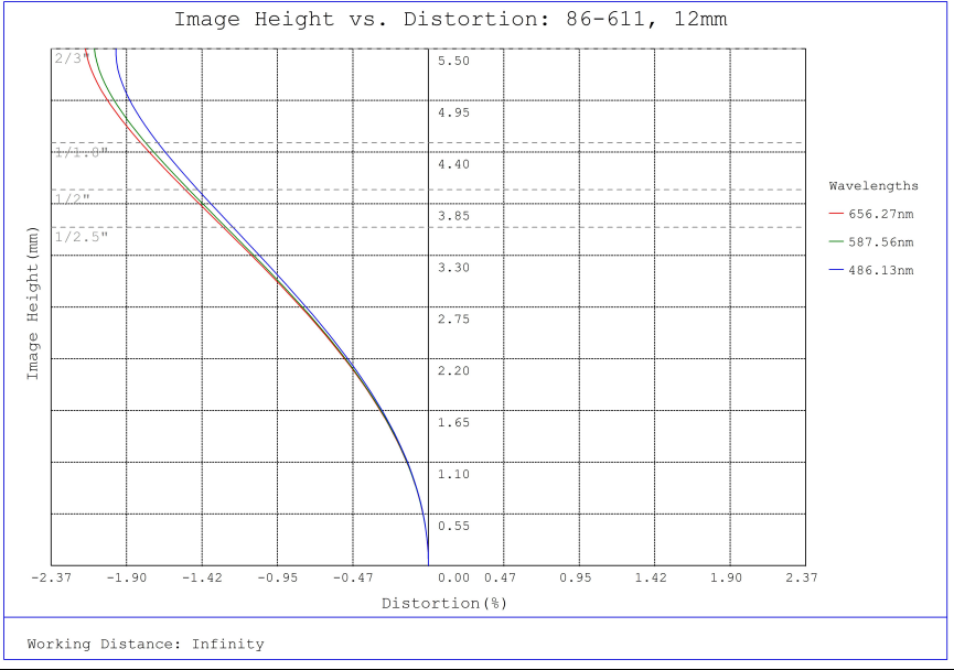
#86-611, 12mm, f/8 Ci Series Fixed Focal Length Lens, Distortion Plot
