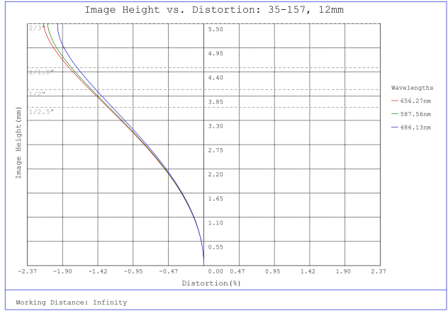
#35-157, 12mm, f/4 Cr Series Fixed Focal Length Lens, Distortion Plot
