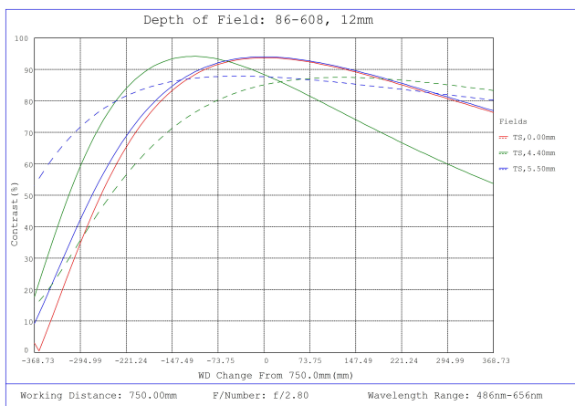
#86-608, 12mm, f/2.8 Ci Series Fixed Focal Length Lens, Depth of Field Plot, 750mm Working Distance, f2.8
