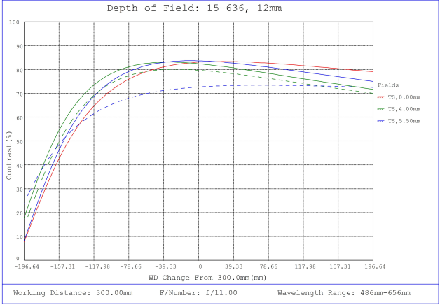
#15-636, 12mm, f/11 Cw Series Fixed Focal Length Lens, Depth of Field Plot, 300mm Working Distance, f11
