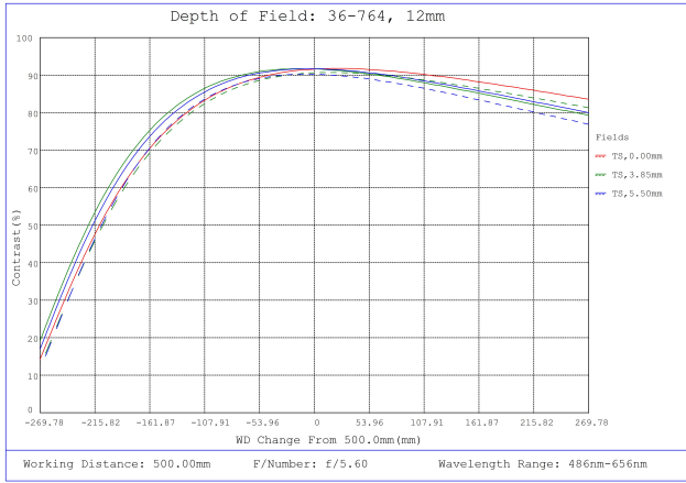
#36-764, 12mm f/5.6, 400-2000mm Primary WD, HRI Series Fixed Focal Length Lens, Depth of Field Plot, 500mm Working Distance, f5.6
