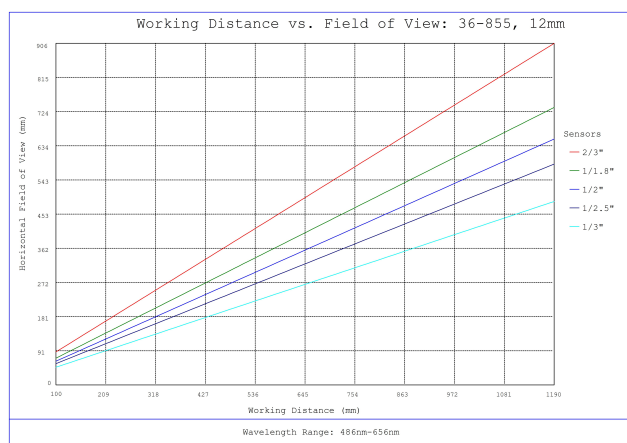
#36-855, 12mm f/5.6, 150-500mm Primary WD, HRr Series Fixed Focal Length Lens, Working Distance versus Field of View Plot
