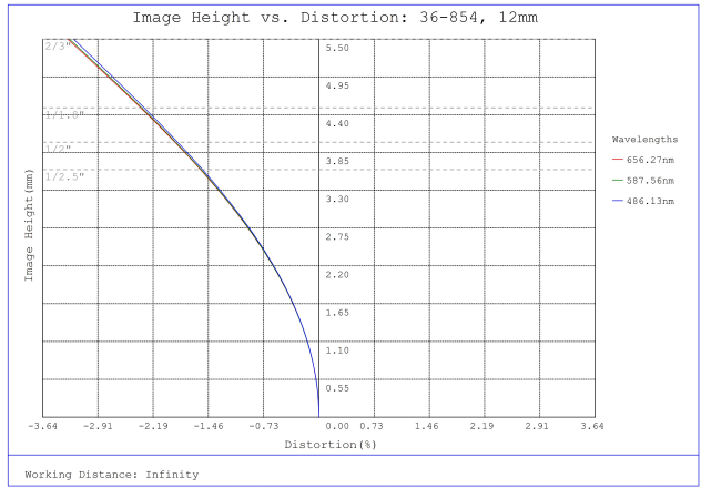
#36-854, 12mm f/4, 1000mm-∞ Primary WD, HRr Series Fixed Focal Length Lens, Distortion Plot
