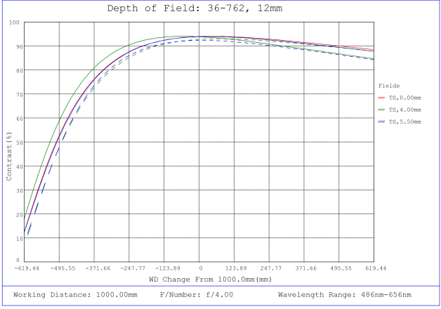
#36-762, 12mm f/4, 1000mm-∞ Primary WD, HRi Series Fixed Focal Length Lens, Depth of Field Plot, 1000mm Working Distance, f4
