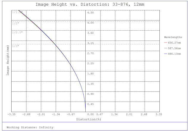
#33-876, 12mm, f/1.8 UCi Series Fixed Focal Length Lens, Distortion Plot
