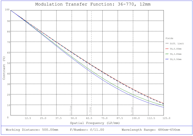
#36-770, 12mm f/11, 400-2000mm Primary WD, HRi Series Fixed Focal Length Lens, Modulated Transfer Function (MTF) Plot, 500mm Working Distance, f11
