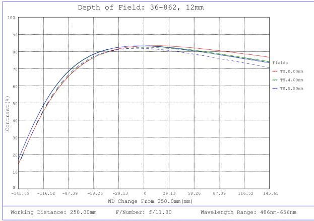
#36-862, 12mm f/11, 150-500mm Primary WD, HRr Series Fixed Focal Length Lens, Depth of Field Plot, 250mm Working Distance, f11
