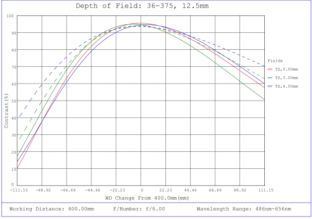
#36-375, 12.5mm FL f/8, Rugged Blue Series M12 Lens, Depth of Field Plot, 400mm Working Distance, f8
