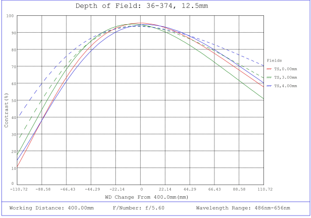
#36-374, 12.5mm FL f/5.6, Rugged Blue Series M12 Lens, Depth of Field Plot, 400mm Working Distance, f5.6
