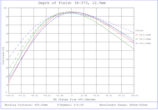
#36-373, 12.5mm FL f/4, Rugged Blue Series M12 Lens, Depth of Field Plot, 400mm Working Distance, f4
