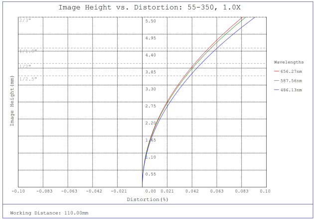
#55-350, 1.0X 2/3" GoldTL™ Telecentric Lens, Distortion Plot
