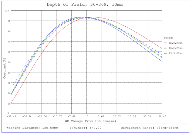
#36-369, 10mm FL f/4, Rugged Blue Series M12 Lens, Depth of Field Plot, 150mm Working Distance, f4
