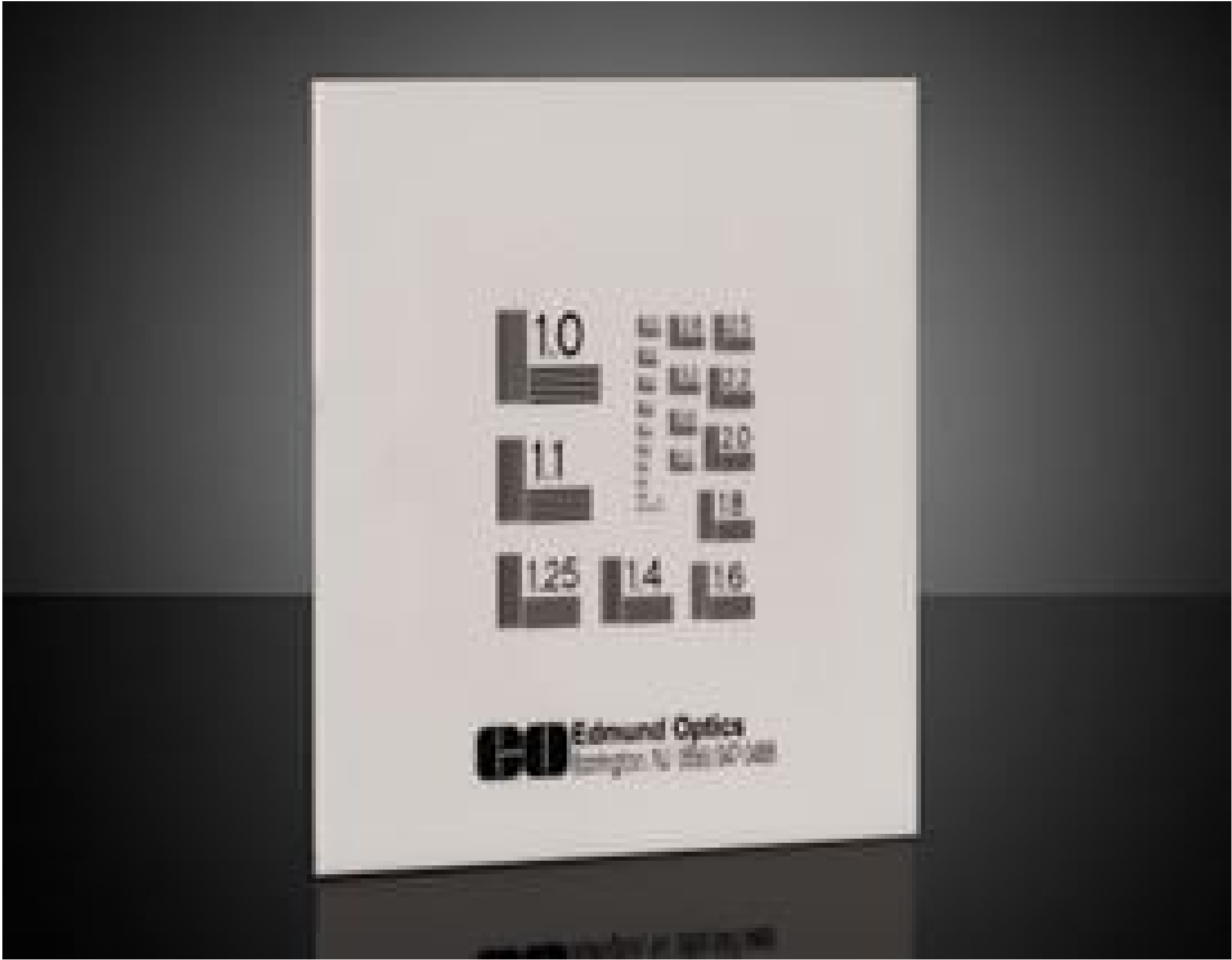
NBS 1963A Resolution Target
