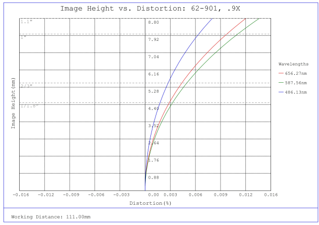
#62-901, 0.9X CobaltTL Telecentric Lens, Distortion Plot
