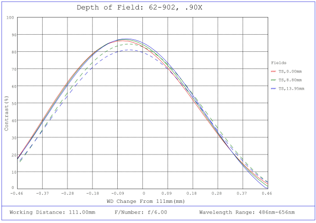
#62-902, 0.9X, 28.7mm F-Mount PlatinumTL™ Telecentric Lens, Depth of Field Plot, 111mm Working Distance, f6
