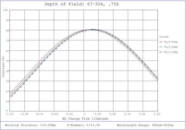
#67-304, 0.75X, 110mm WD, In-Line CompactTL™ Telecentric Lens, Depth of Field Plot, 110mm Working Distance, f13.3
