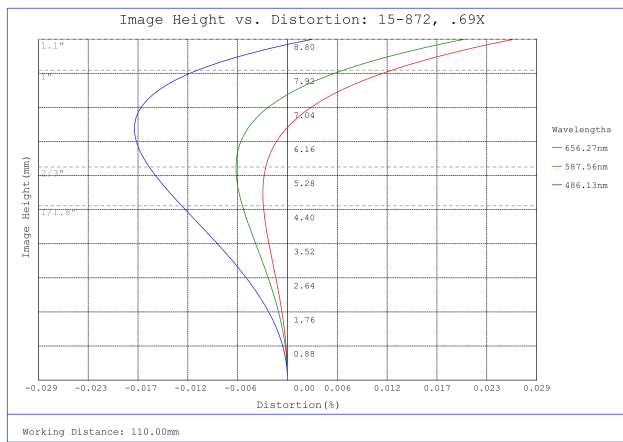
#15-872, 0.69X Cobalt TL Telecentric Lens, Distortion Plot
