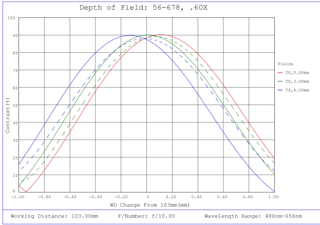
#56-678, 0.60X SilverTL™ Telecentric Lens, Depth of Field Plot, 103mm Working Distance, f10
