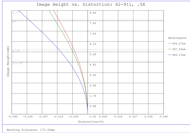
#62-911, 0.5X Cobalt TL Telecentric Lens, Distortion Plot
